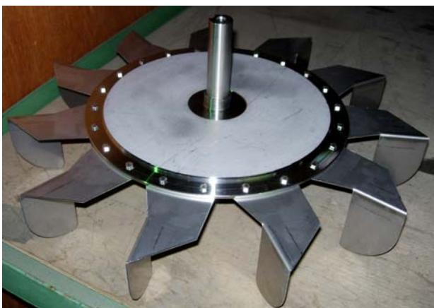
A complete main shaft, flywheel and impeller assembly:
