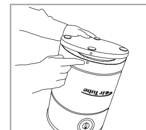
Step 8 Place lid back to its proper position by aligning screw holes.
