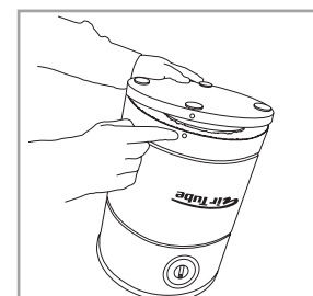
Step 8 Place lid back to its proper position by aligning screw holes.
