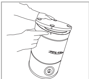
Step 7 Place lid back to its proper position by aligning screw holes.
