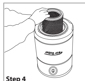
Step 4 First remove HEPA filter by placing your hand on the inner side of the filter. Then pull up gently until totally out.
