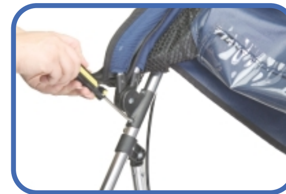
1 Using a phillips head screwdriver, screw brackets to Jogger frame.
